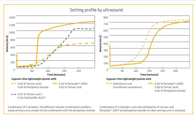
Gypsum plaster or gypsum-lime plaster is at present the most frequently used interior plaster. Easy application and a consistent setting behaviour are critical for the success of the user. Retardan®-200 P is especially suitable as a setting regulator for use in gypsum plaster due to its large pH-value tolerance. It can be optimally combined with other retarders e. g. fruit acids.
