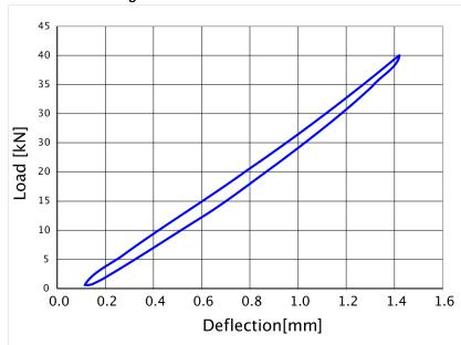
Static stiffness analogous to DIN 45673-1. Dimensions of test specimen:  $360 \times 160 \times 25$  mm; Spring index: c = 29 kN/mm, determined as per the secant method between 8 kN and 32 kN.
