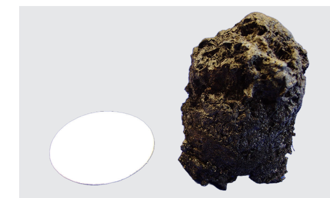
Foamed-up Interdens® Type 15 sheet: At a temperature of approx. 150 °C, Interdens® Type 15 begins to expand to many times its original volume
