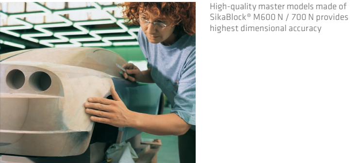
Models milled out of SikaBlock® PROLAB 65 N fulfil highest demands of surface quality
