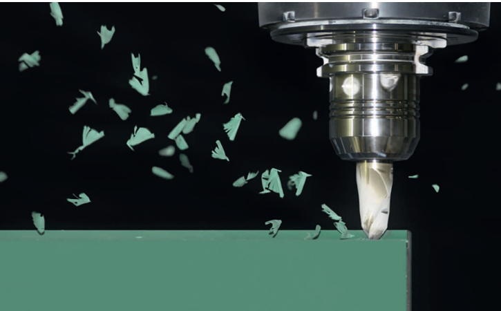
SikaBlock® M945 provides excellent milling behaviour with low dust formation
