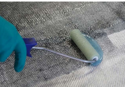
Wet lay-up with SikaBiresin CR168
