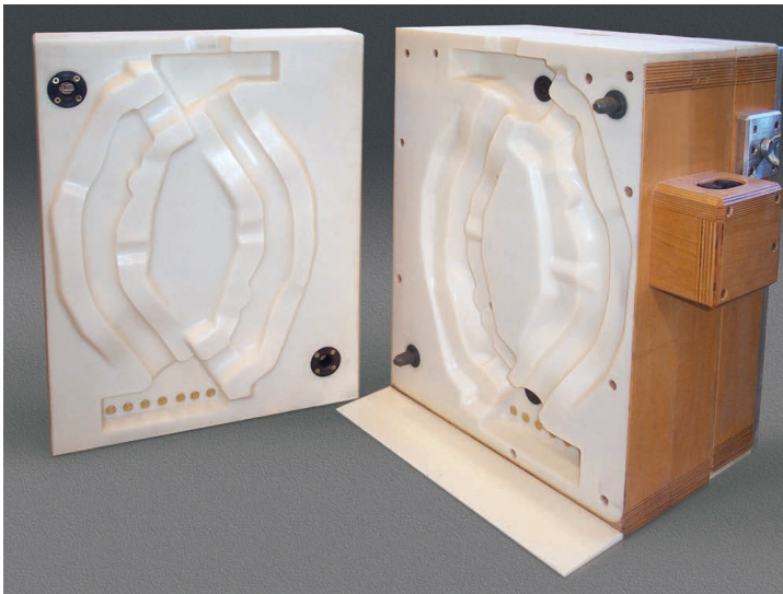
Core box made of SikaBiresin® UR132
