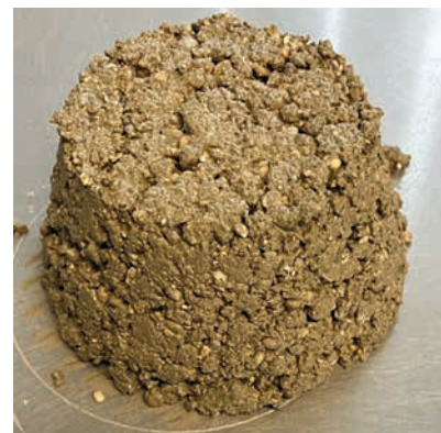
Image 1: Left: w/c = 0.6 The mortar is still compact and has a light, shiny water film.
