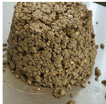
Right: w/c = 0.55 The mortar cake falls apart slightly and looks very dry and brittle.
