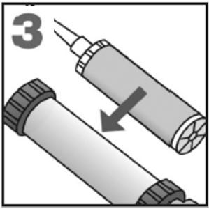
Pressing on the cartridge shortly until uniform coloured material comes out (approx. 1 cm). Start application by putty or brush.
