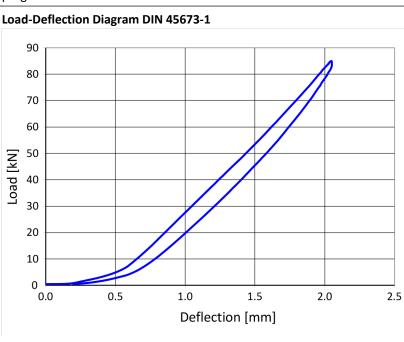
Dimensions of test specimen  $360 \times 160 \times 25$  mm; static stiffness analogous to DIN 45673-1.
