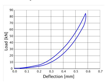
Static stiffness determined according to DIN 45673-1. Dimensions of test specimen  $360 \times 160 \times 25$  mm; Spring index k<sub>stat</sub> = 222 kN/mm (±10 %), determined as per the secant method between 17 kN and 68 kN.
