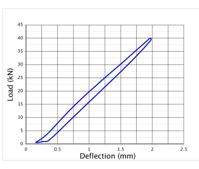
Static stiffness determined according to DIN 45673-1. Dimensions of test specimen  $1000 \times 180 \times 25$  mm. Spring index k<sub>stat</sub> = 25 kN/mm (±10 %), determined as per the secant method between 4 kN and 32 kN.
