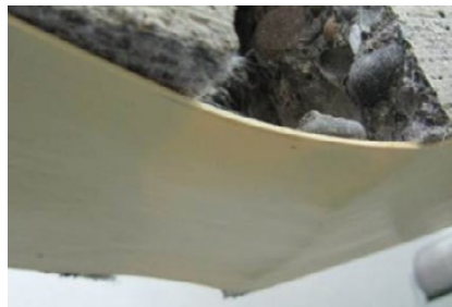
Elongation and crack bridging capability illustrated with a flexural tensile test (in overview and close-up)
