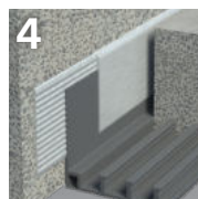
4 Connection joints to existing components
