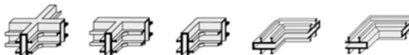
Cross piece vertical T-piece vertical L-piece vertical L cross piece flat L-piece flat, coverslab inside
